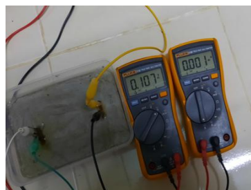
Fig. 2: Electricity supply test for the mortar-based cell connected to a resistor
